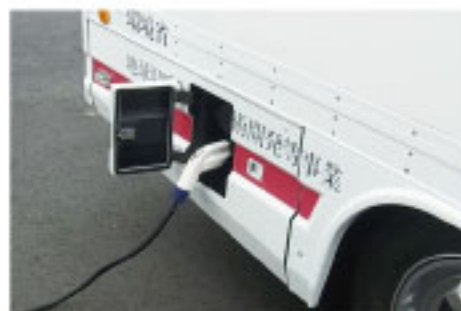
急速充電及び普通充電(写真)対応 Corresponds to rapid charging & regular charging (as shown)
